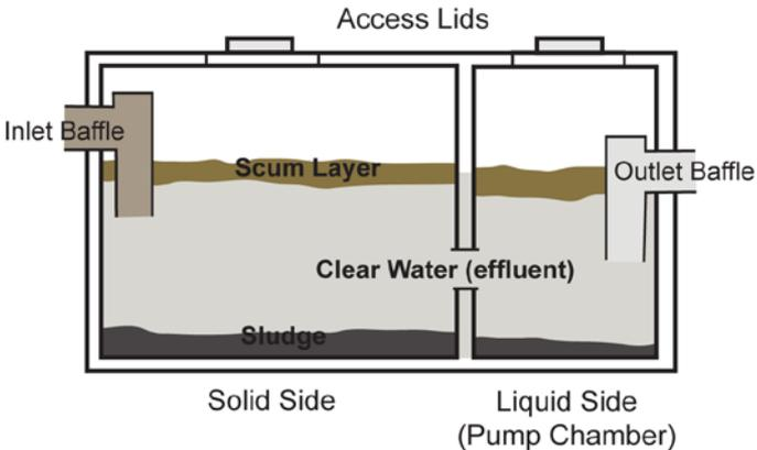
The waste water entering the septic tank separates into 3 layers
